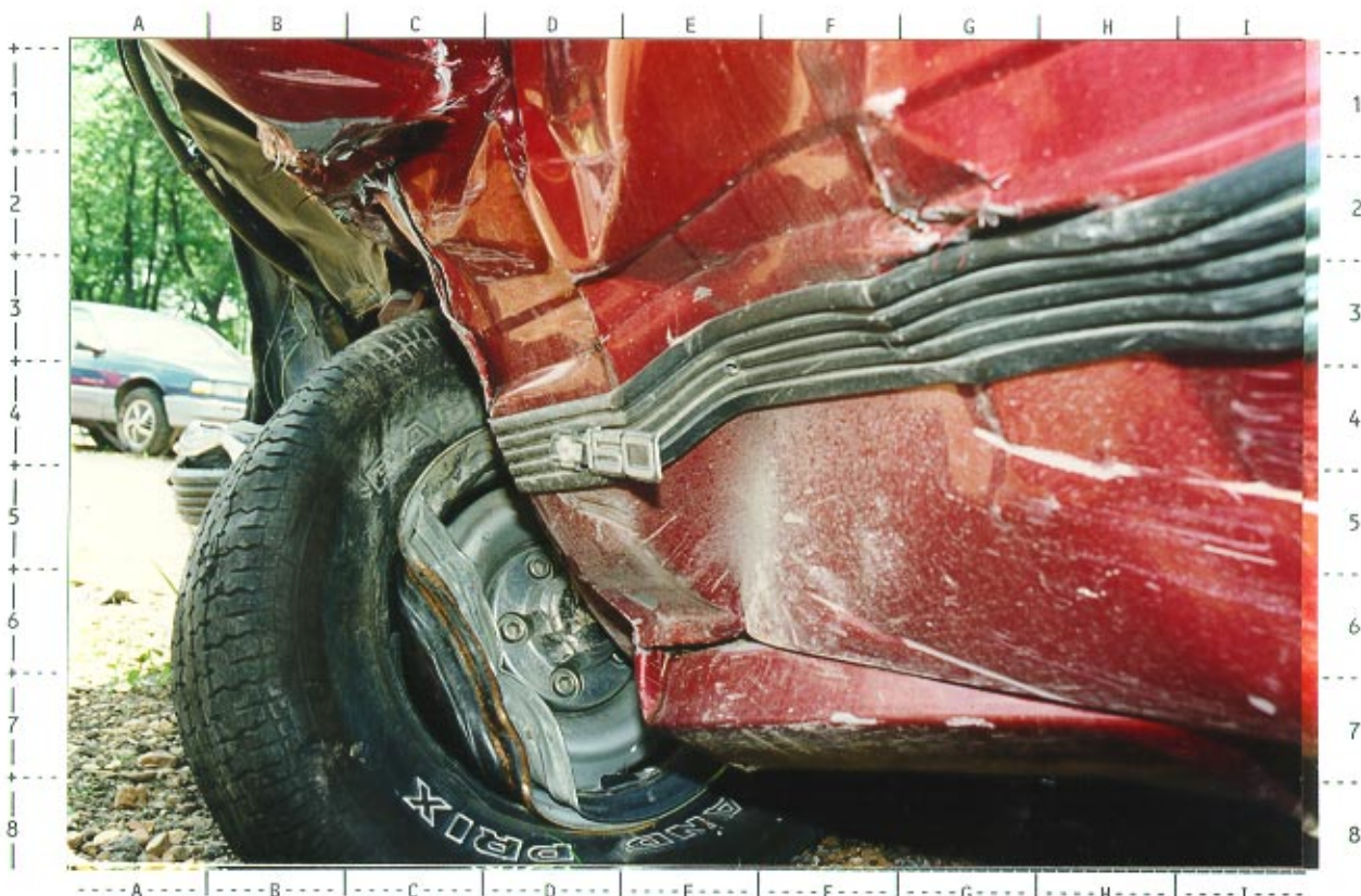
# 70 -- Close-up of direct damage to 1988 Chevrolet pickup's LF rim and also behind displaced left front wheel--viewed from back left
